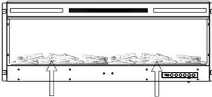
5. Once completed installing the crystal embers or the fire log, reinstall glass panel. The hooks on the back of the glass panels fit into the slots on the side of the firebox. Once in the slots, the glass panel goes down and locks into place.
