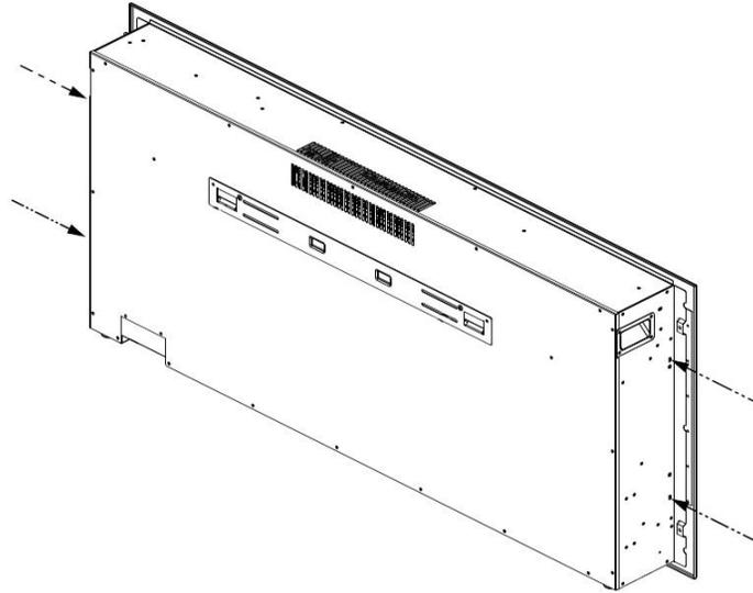
*Note: The side screws are for securing the front panel to the fireplace during shipping and do not need to be reinstalled.*
