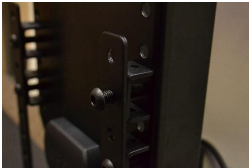
Thread bolt through bracket and spacer
