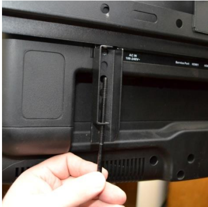
Install mounting screw in holders on TV bracket
