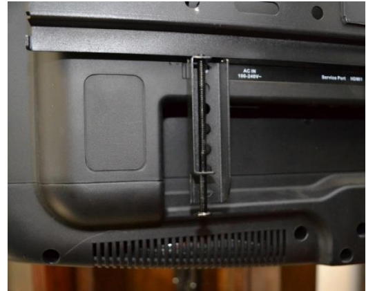
Tighten screw so that it is finger-tight to the swivel bracket
