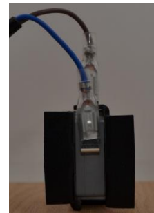
Connect Blue Wire To Bottom Connection
