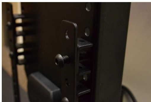
Thread bolt through bracket and spacer
