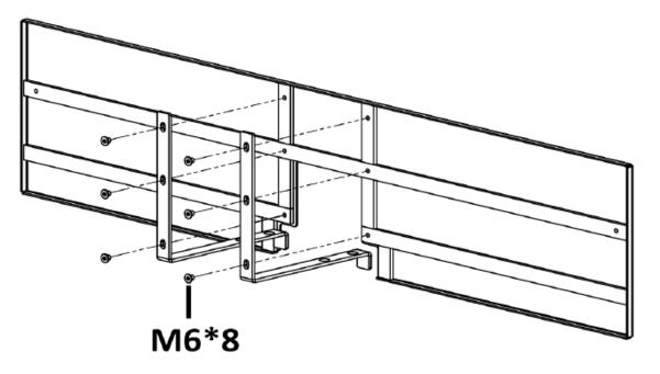
2. Attach the U bracket to the L brackets using 2 M6x16 screws per bracket.
