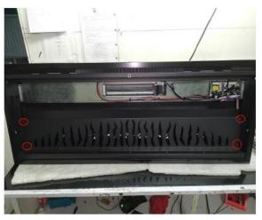
10. Once the flame panel is installed, reinstall the flame display board and the bar holding the bar in place.
