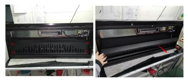
7. After removing the flame panel, locate the flame rod motor. The flame rod should be attached to the motor.
