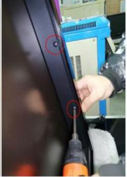
4. Remove the 4 screws holding the bar at the top of the flame display board.
