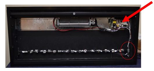
7. Disconnect the HEAT1, HEAT2, and FAN cables from the control board
