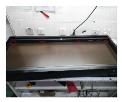
5. Once the bar is removed, remove the flame display board.
