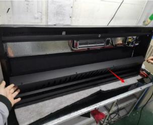
7. After removing the flame panel, lubricate the 2 rubber grommets holding the flame rod in place.
