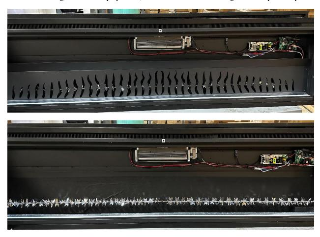
7. After removing the flame panel, locate the flame rod motor. The flame rod should be attached to the motor.
