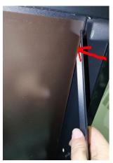
18. Reinstall the bar at the top of the flame display panel.
