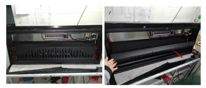
7. After removing the flame panel, locate the flame motor and check the coupler between the flame rod and the flame rod motor.
