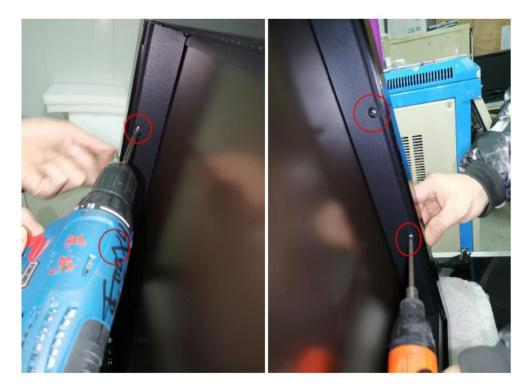
17. Once the side panels are reinstalled, reinstall the log/crystals and front glass panel.
