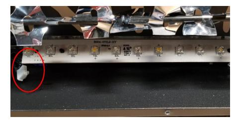
10. After the cable is disconnected, remove the defective LED light strip from the fireplace. To remove, pinch the clips holding the LED light strip in place and lift the LED light strip up to remove.
