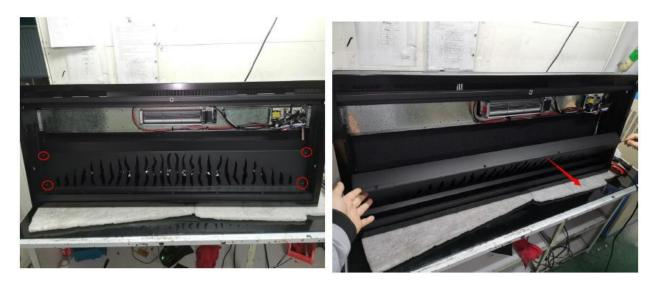
7. Once the unit is open, locate the LED Light strips
