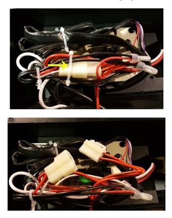
8. After disconnecting the motor cable, remove the flame rod and motor from the fireplace.
