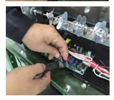
5. Install the back cover and fix it using screws.
