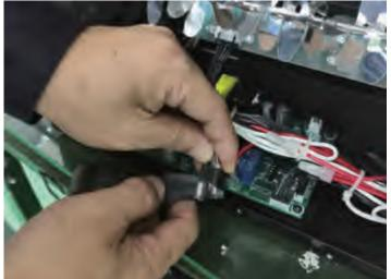
Wrap the three wires together using electrical tape.
