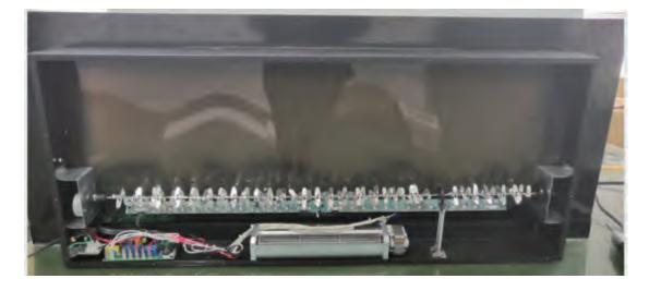
3. Disconnect the three wires of HOT1, HOT2 and FAN as below.
