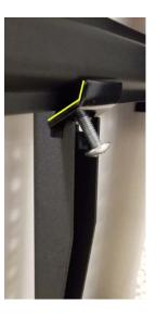
4. With a Philips-head screwdriver, tighten the screw so that the screw is tight against the cross bracket, as shown in the picture below.
