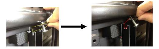
4. With a Philips-head screwdriver, tighten the screw so that the screw is tight against the cross bracket, as shown in the picture below.
