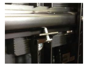
5. After installing the first locking bracket, install the 2<sup>nd</sup> locking bracket on the other TV bracket in the same manner. Your TV should now be locked in place and not move from side to side.
