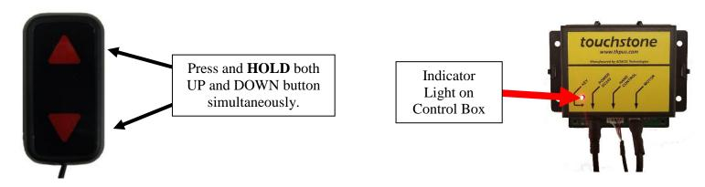
2. Release the UP and DOWN button and the indicator light on the top of the control box will flash 3 times and turn off. The lift will go all the way to the bottom, back up the top and all the way down to the bottom again. The red light on the control box will come back on when the initialization procedure is complete. \*\*Note: Do not proceed until this procedure is complete.
