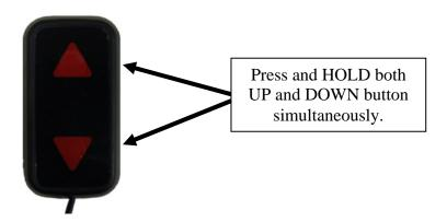
2. Release the UP and DOWN button and the indicator light on the top of the control box will flash 3 times and turn off. The lift will go all the way to the bottom, back up the top and all the way down to the bottom again. The red light on the control box will come back on when the initialization procedure is complete.
