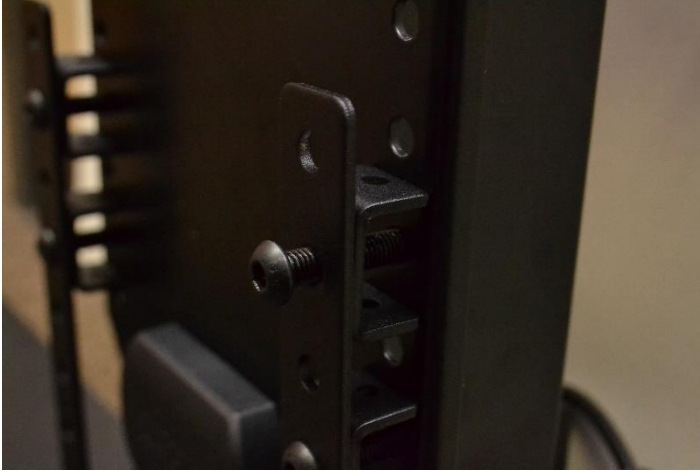
Thread bolt through bracket and spacer
