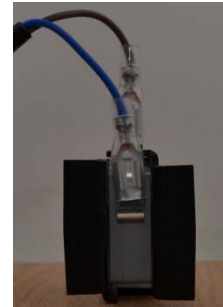
Connect Blue Wire To Bottom Connection
