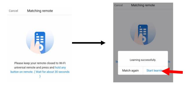
13. Once the Start Learning button is pressed, you have 30 seconds to pair a button on the SRV/ValueLine Wireless RF remote to the app. To pair the UP button, press the UP button on the SRV/ValueLine Wireless RF remote to pair the button to the app. Press the "clover" button in the app to test the function. The lift should go UP.
