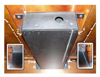
6. Remove the lift from the cabinet (either you can lift it through the top of the cabinet or slide it out one of the rear access panels, if your cabinet has rear access panels).
