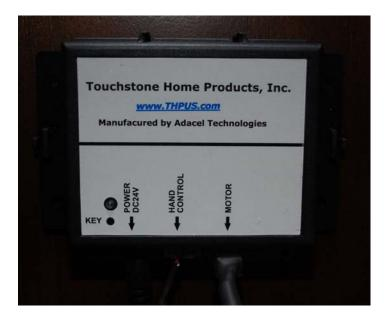
2. With a straightened out paper clip, push it into the hole and hold for 3 seconds until the indicator light flashes twice and turns on solid red.
