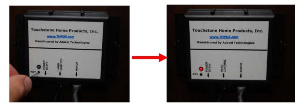
3. Press any button on the wireless remote to match the remote with the control box. If you are successful, the red light on the control box will turn off. If the pairing fails, the indicator light will flash 4-5 times.
