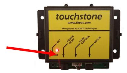
2. With a straightened out paper clip, push the paper clip into the hole and hold for 3 seconds until the indicator light on the control box turns OFF.
