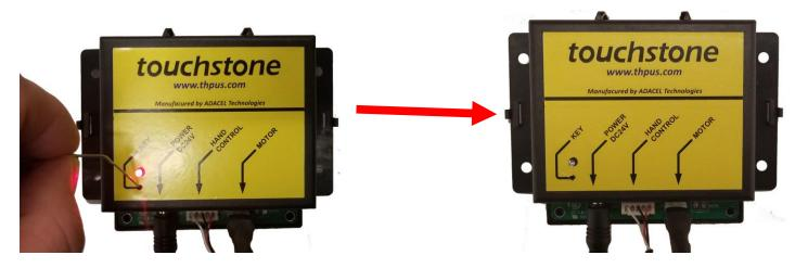
3. Press any button (UP, DOWN, or STOP) on the WIRELESS REMOTE to pair the remote control to the control box. If you are successful, the red light on the control box will flash 3 times and turn ON solid RED. The wireless remote control is now paired to the lift.
